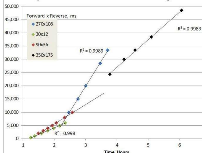
By varying the duration and ratio of forward and reverse voltage pulses, the BluePippin can resolve and purify DNAs between 1 and 50kb. The BluePippin can also be used in constant field DC mode like the original Pippin Prep for DNA fractionations between 50 and 1500bp.
