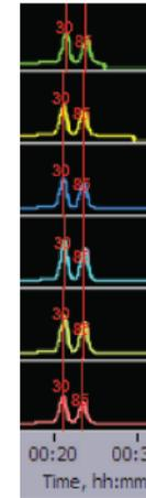
Extracted samples are run on an Agilent Bioanalyzer using a DNA 1000 chip. The analysis volume is 3 µl from a 30 µl elution volume (1:10 dilution). The following bioanalyzer results indicate typical results from QC testing:
