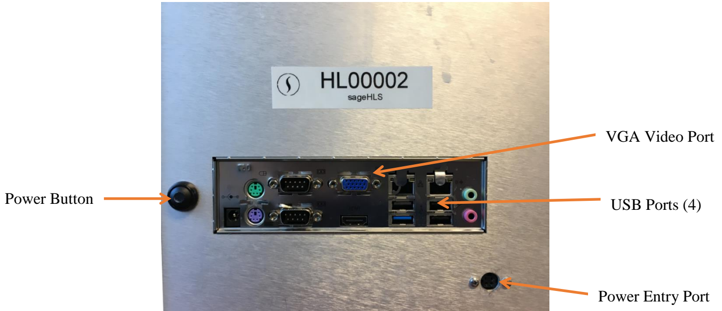
Figure 3.1. Rear Panel of the SageHLS
